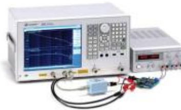
Pomona 3787-C-18 test lead (connected to gain-phase receiver ports) Pomona 2885 BNC breakout (connected to 0017CC)
