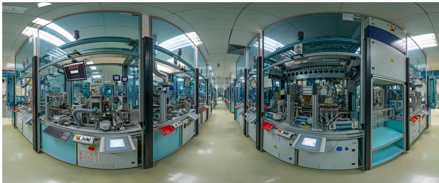
360° panoramic view of a typical automated production line for TE Connectivity general purpose power relays.
