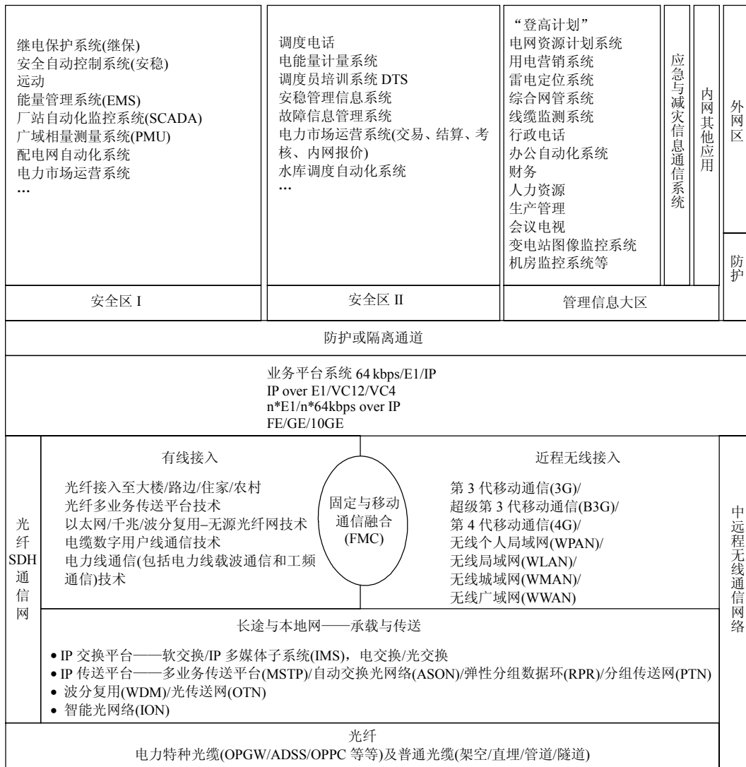
图 1 智能电网的信息通信保障体系框架 Fig. 1 Guaranteeing system structure of China national smart grid
